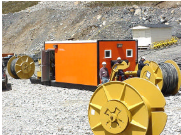
Portable Cable Repair Station @ Compania Minera Antamina SA, Peru
